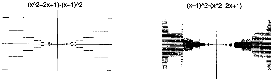
Figure 10: The bow tie monster plotted with MAPLE 6. Changing the order of calculation of the two terms leads to a surprisingly different appearance for the monster. For the sake of clarity the axes labels are omitted. All magnitudes correspond to those given in figure 6.
