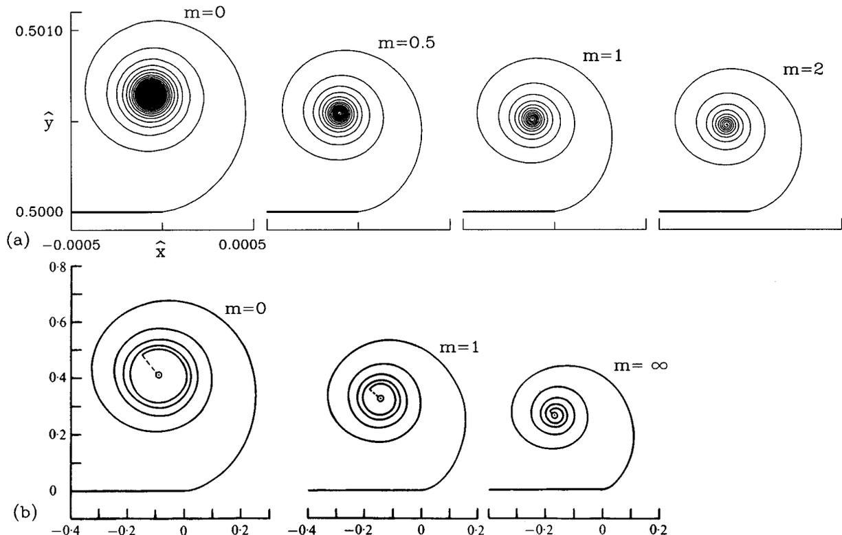
FIG. 8. (a) Computed solution at  $\hat{t}=0.0002$ , with  $\delta=0.00004$  and the indicated values of  $m$ . (b) Pullin's solution for the self-similar planar roll-up at the edge of a plate (reproduced from Pullin<sup>2</sup>).
