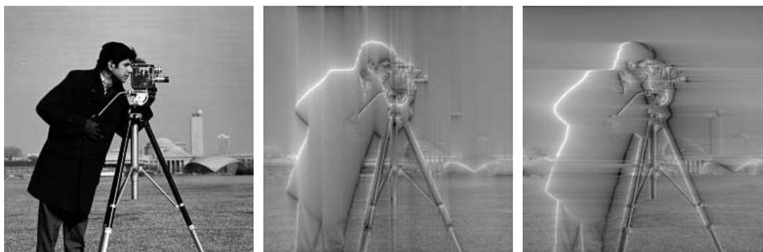
**Fig. 5:** Edge detection in image processing using the DHT. The left image is the original image, the center image is the edge enhanced image along the vertical direction and the right image is the edge enhanced image along the horizontal direction.
