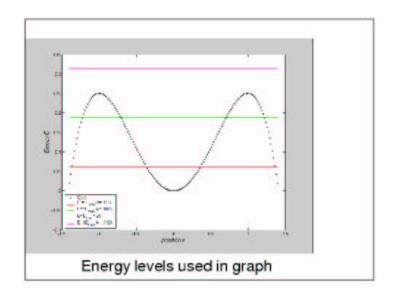
Plot of G(x) together with several energy "levels". Given a value of E, a phase orbit with that energy can only exist for positions where  $G(x) \leq E$ . Since the difference
