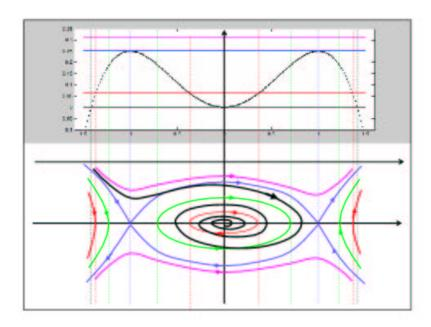
Using the potential energy diagram to draw the phase plot. The vertical axis on the bottom graph is velocity, while at the top total energy. The horizontal axis is displacement.
